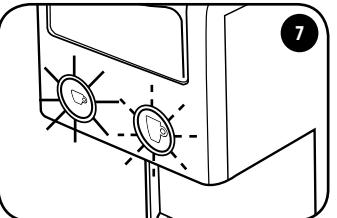
At the end of the descaling cycle, the button is steady on while the button is flashing.
